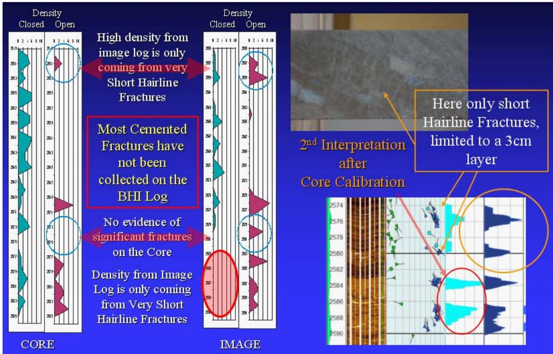
Figure 11 Comparison of original BHI and core interpretation, and revised BHI log after reviewing the BHI in the light of data from core.
