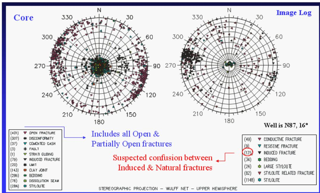
Figure 5 Core Stereonet Plot shows all open & partially open fractures. On BHI, 1148 Stylolites were not plotted to make the diagram clearer because those Stylolites features were confused with all other sedimentary and fracture features.
