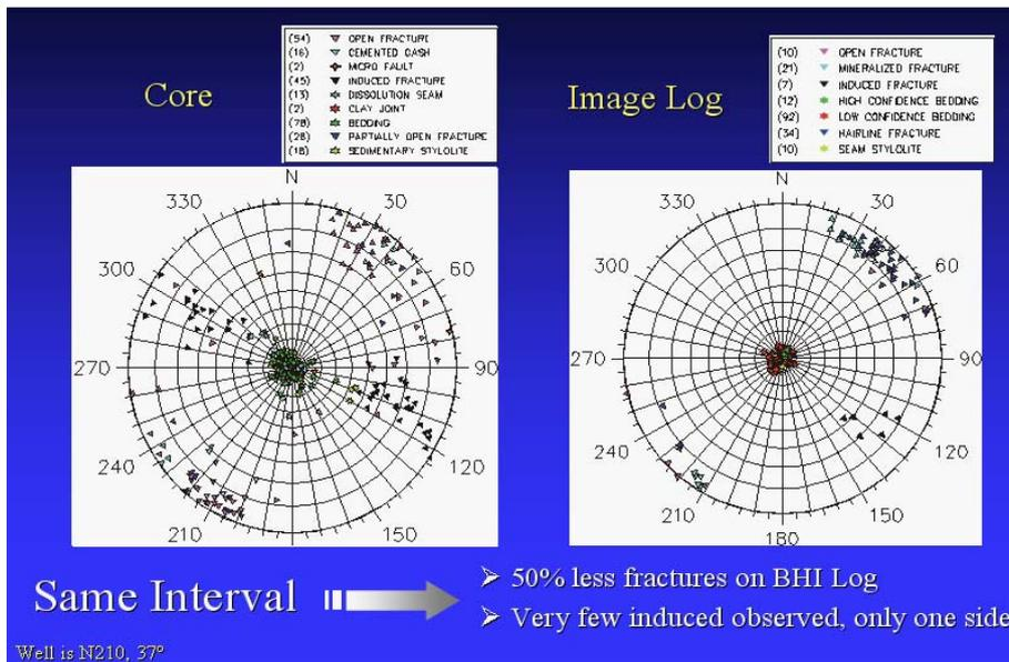
Figure 3 Stereonet Plot - Case #2
