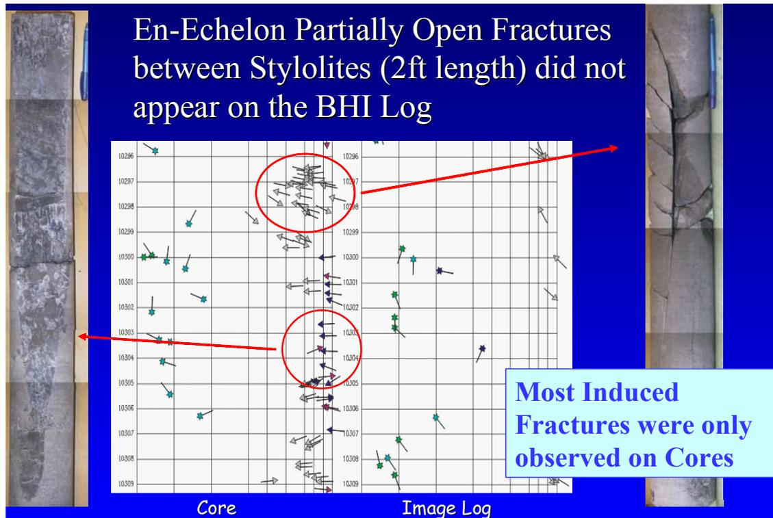
Figure 10 Photo on left side shows partially open fracture with Calcite (white) filling.
