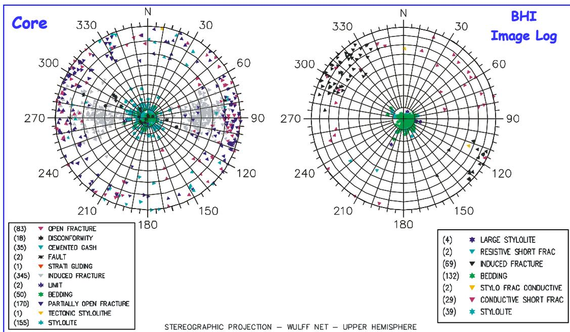
Figure 9 Stereonet plots – Core & BHI Log.
